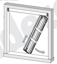
Placing the Pietta 22 main body to the left Using a spirit level place the Pietta 22 main body to a perfect vertical position
