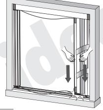
Push the sliding guide downwardly until the bulges engage within the lower guide.
