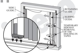
Placement of the sliding guide into the lower guide.
